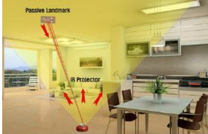
Schematic showing localization principle by StarGazer™
